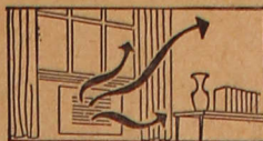
Wall panel heaters have heating coils behind a decorative grill. Small fans may be used with this thermostatically controlled unit.
