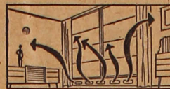
Baseboard units heat by both radiation and convection. All surfaces are warmed evenly, and control is by individual room thermostat.
