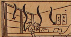
Ceiling cable heat is invisible. Wires less than 1/8" thick are fastened to ceilings before plastering. Each room can have a thermostat.
